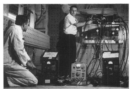
BILL PUTNAM, left, and Larry Woolrich prepare a test which will duplicate aerodynamic forces on the fin of a test vehicle. Larry is adjusting one of the hydraulic cylinders which will exert force.
